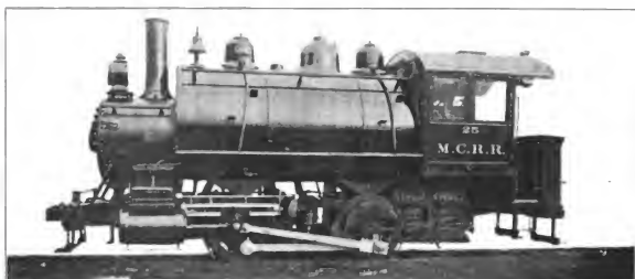
Fig. 3. Four-Wheel (0—4—0) Tank Switching Locomotive. Built by the American Locomotive Co. for the Michigan Central. Cylinders 18 in. x 24 in., Working Steam Pressure 180 lbs. per sq. in., Heating Surface 1,308 sq. ft., Diameter of Drivers 52 in., Weight on Drivers 114,400 lbs., Total Weight 114,400 lbs.
